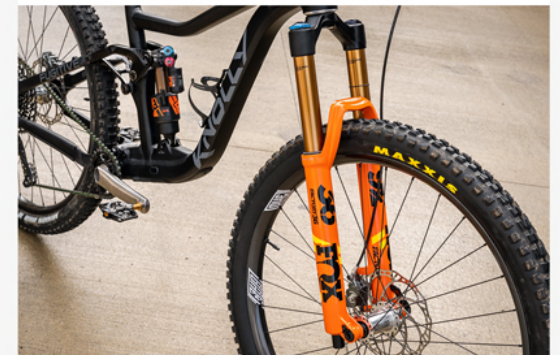
Warren's size medium Fugitive is a no-holds-barred build. The fork is the Fox Factory 36 GRIP2 but has something different than most.
